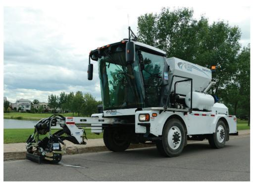
SuperiorRoads Solutions offers two models of pothole patchers - the Python 5000 and the SR 6000. They are unique, one-person operated pothole patchers that repair an average pothole in less than two minutes using standard asphalt mixes.
